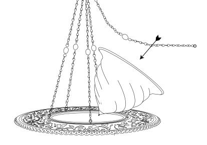
${f B}_{f \cdot}$  Insert the lampshade through the chains as shown in the picture.
