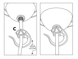
Install bulb. Do not exceed the maximum wattage for this fixture.
