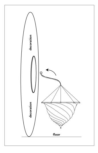
**B**. Pass suspension strings through the central hole of the flat disk and gently pull strings to place the small shade close to the disk hole
