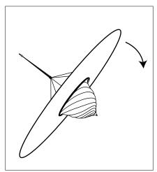
**D**. After the installation of the fixture and electrical connections hang the lamp to the hook of the ceiling canopy. Hook the tassel.
