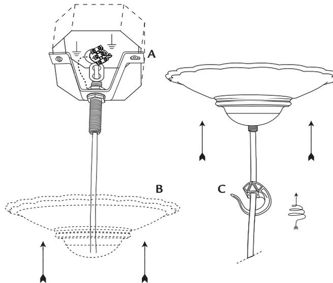
5. Screw the hook **C** onto the nipple and tighten securely.
