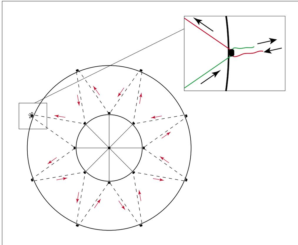
10. Hang the hook of the glass drop into the ring of the small disk.
