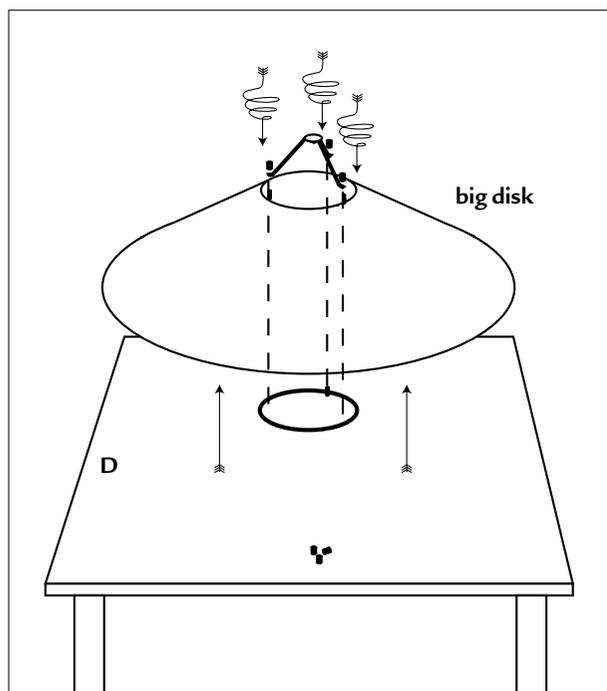
8. Insert element **E** and tighten the three screws on element **D**.
